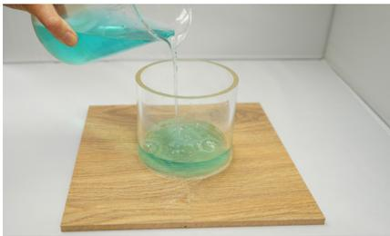
**Test 1:** a test with a cylinder filled with water that is put on the joints of an installed floor for 24h
