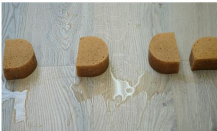
**Test 2:** a sponge test with wet sponges on the joints of an installed floor for 24h.
