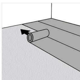
**1. Underlay:** The installation starts with a BerryAlloc underlay with integrated moisture barrier. Use the **BerryAlloc Excellence Impact+** or the **Excellence Plus** underlay for the best result. Read the *BerryAlloc Underlay guide* for more info. Even if the laminate is water resistant, a moisture barrier is necessary!
